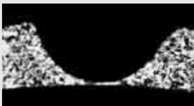
Fig. B.1: Pitting corrosion on a cold strip made of austenitic steel. Sectional view enlarged 50x
