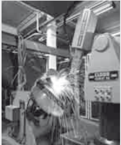
Welding of corrugated hoses
