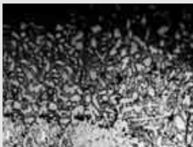
Fig. B.8: Dezincing in a copper-zinc alloy (CuZn 37). Sectional view enlarged 100 x
