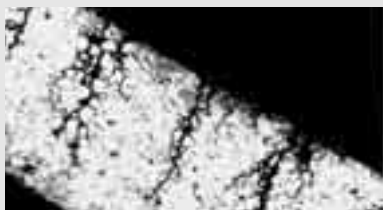
Fig. B.5: Transcrystalline stress corrosion cracking in a cold strip made of austenitic steel. Sectional view enlarged 50x
