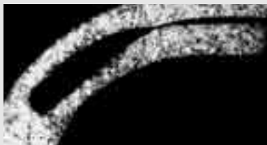
Fig. B.6: Crevice corrosion in a cold strip made of austenitic steel. Sectional view enlarged 50x
