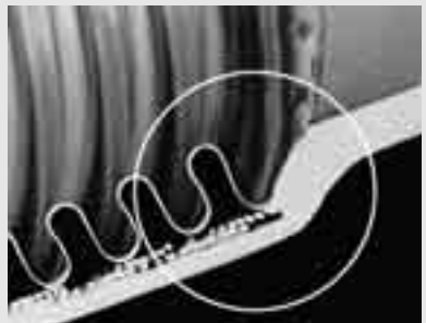
Cross-section of connection fitting complying with the DIN standard and avoiding burrs and crevices.
