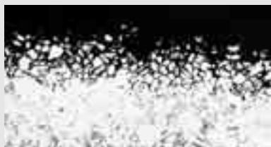
Fig. B.3: Intercrystalline corrosion (grain disintegration) in material 1.4828.
