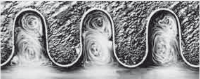
Primary and secondary vortices in the turbulence zone of a HYDRA annularly corrugated hose (factory image).
